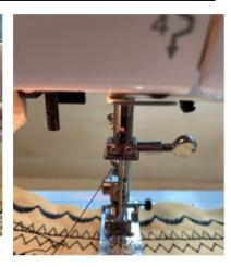
Place the thread on the holder and guide under the plastic hook and down channel 1
