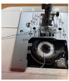
Place the bobbin in the case in an anticlockwise/backwards direction.
